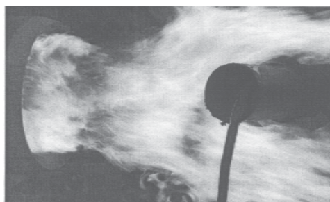
Fig.6 Samples placement for deposition in relation to the mouth of the burner and flame
